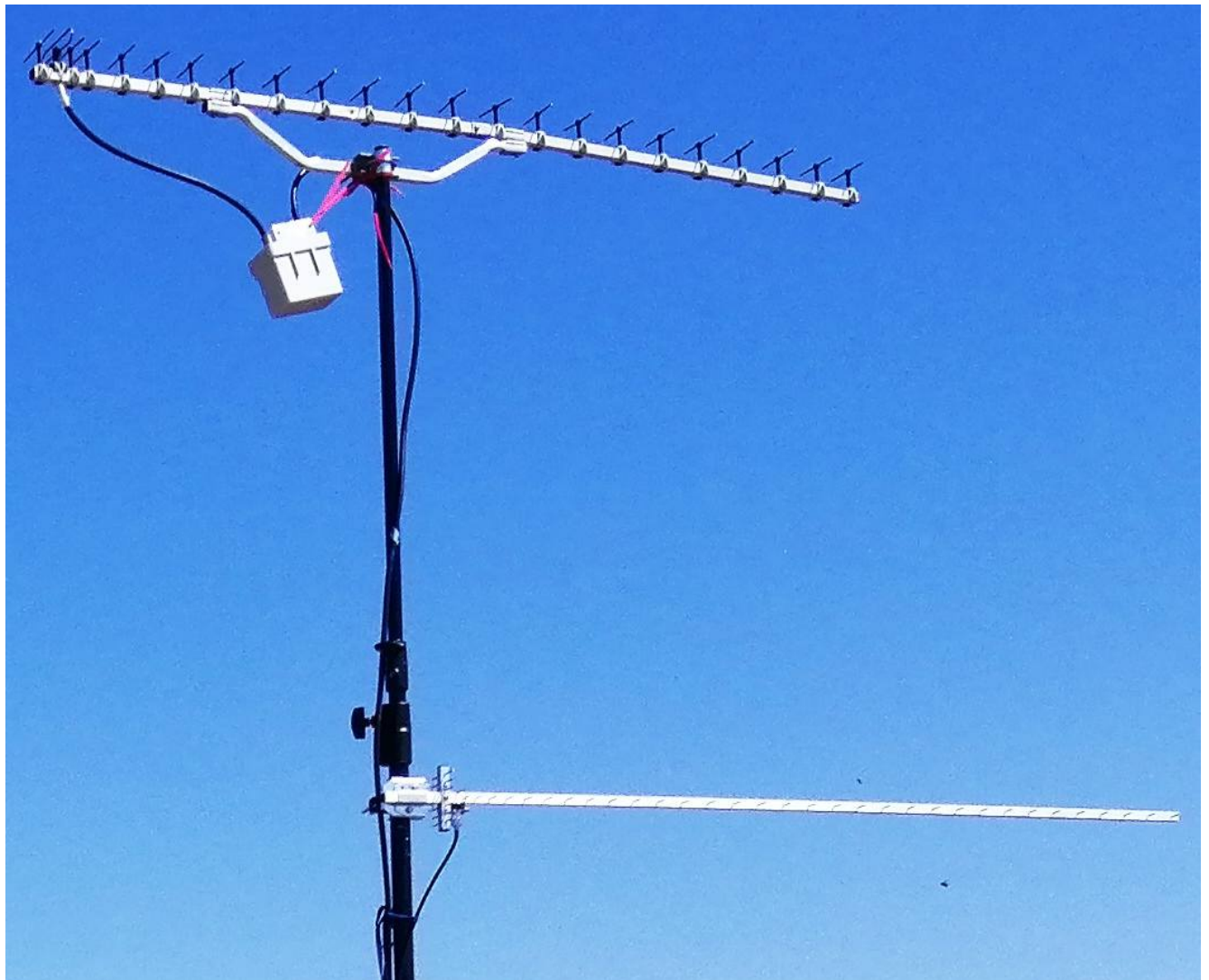
YO3GNF/P KN25EH setup for 23 and 13 cm band
