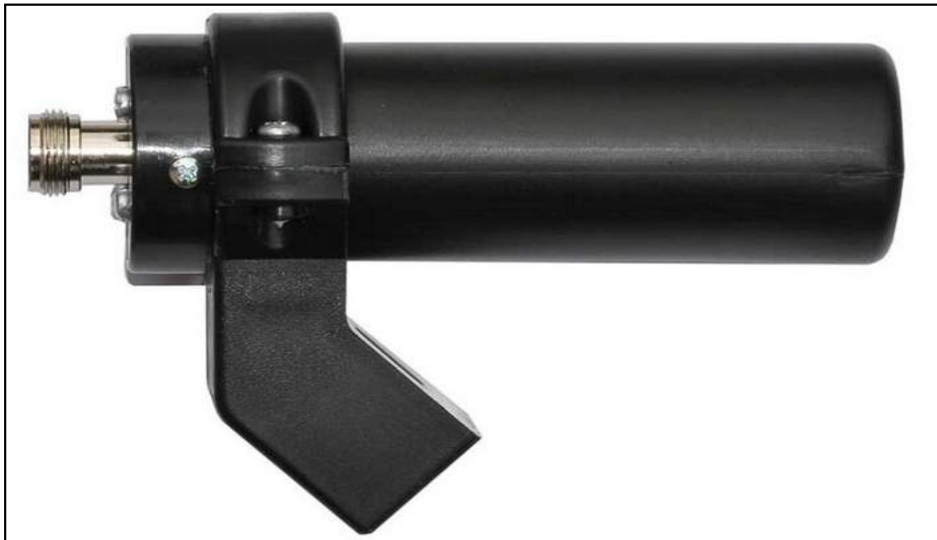
Feed – Illuminator for offset dish with f/d 0.5 – 0.8, QRG: 5.1-5.9 GHz, PWR: 10 Watts,
