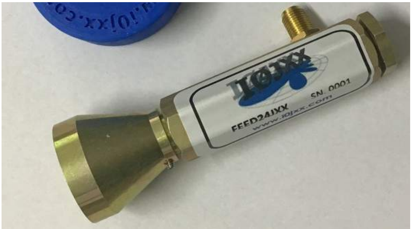
Feeder 24 GHz for OFFS., F/D: 0,6-0,7, PWR: 30W, Quelle: https://www.i0jxx.com/de/24-ghz/274-FEED24JXX.html
