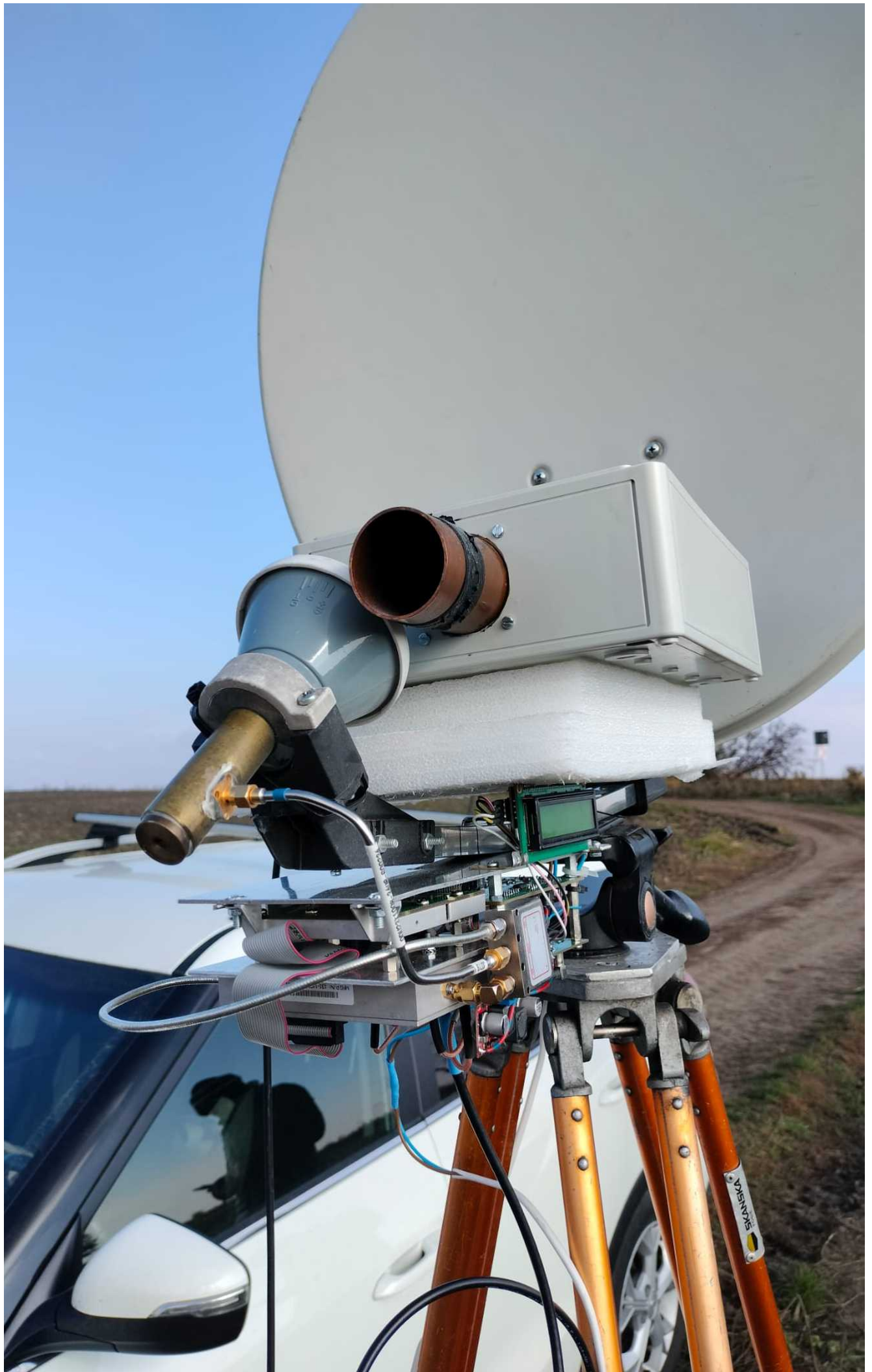
Mihai - (YO8RHM) - Transverter 6cm with SM6FHZ septum feed (circular)
