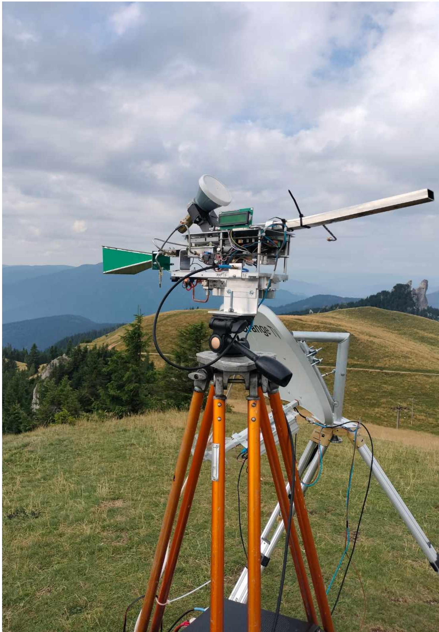
Mihai, YO8RHM (1m agl., 1650m asl.): In the picture my setup for 3cm (front) and 1.2cm (back)
