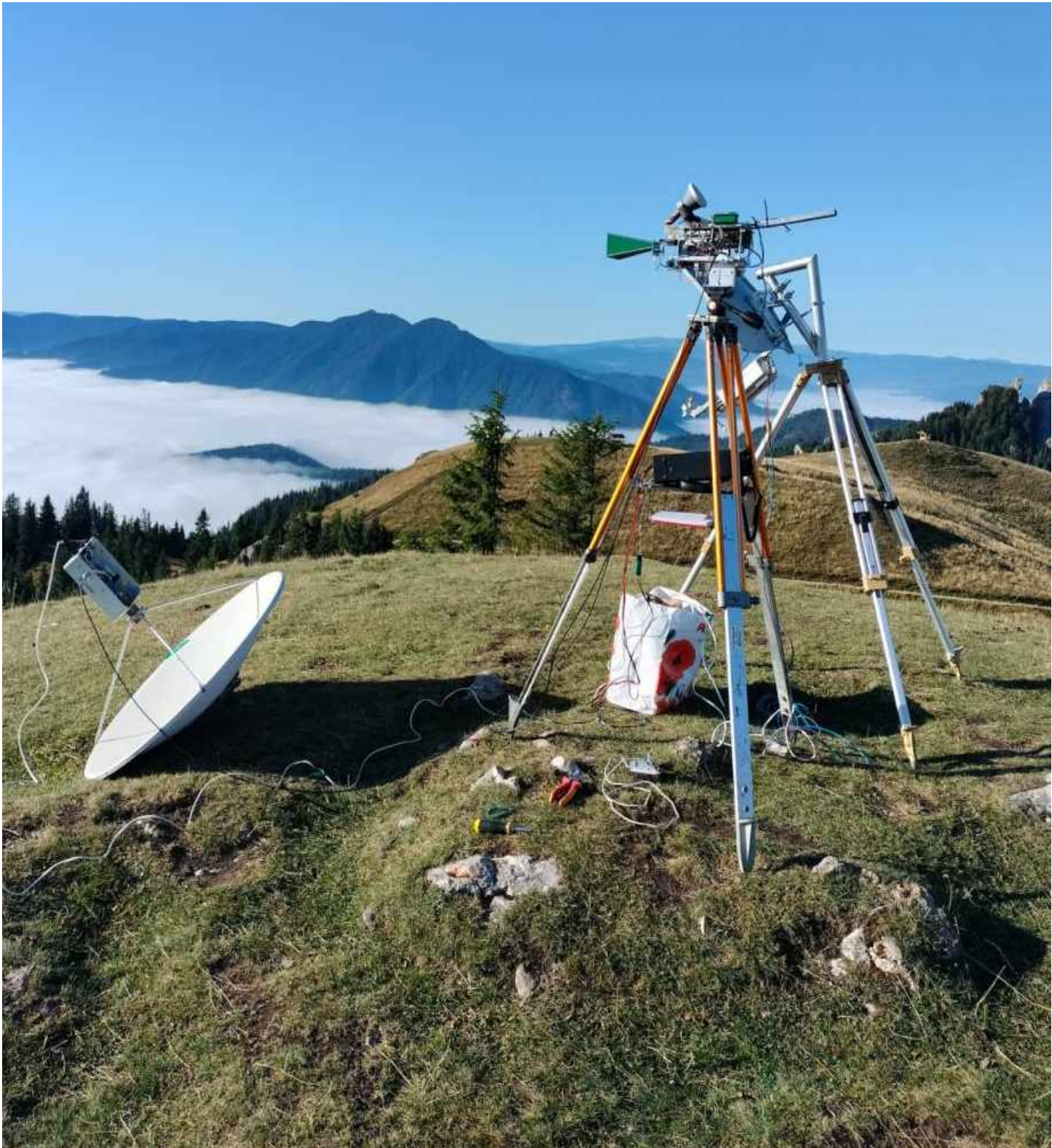
Mihai, YO8RHM: Equipment for 5.7 (1W, prime focus 90cm), 10GHz (9W, horn) and 24Ghz (2W, offset 60cm)
